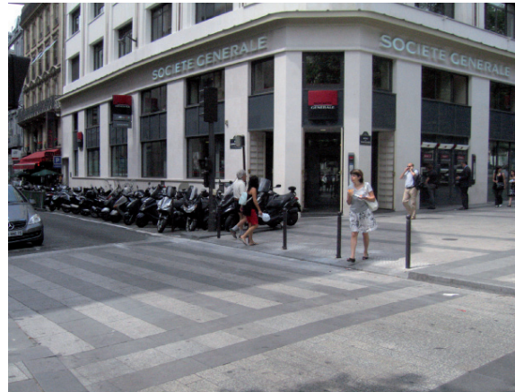
Partly depressed sidewalk for side ensures good accessibility for both pedestrians and vehicular traffic. Paris, France
