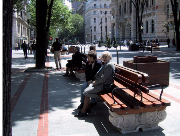
Opportunities to rest should be provided every 100m/330'. Comfortable benches with back and arm rests should be provided. Bilbao, Spain
